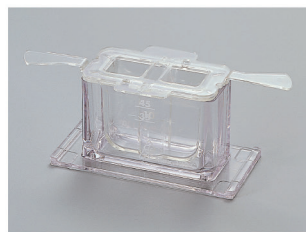
Small sample cup (10ml) Used when measuring small volume samples
